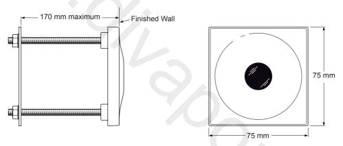
**Note!** The M6 fixing studs supplied allow the LR sensor to be attached through a wall to a maximum thickness of 165 mm. If longer M6 fixing studs are required, these will have to be purchased through your local supplier.
