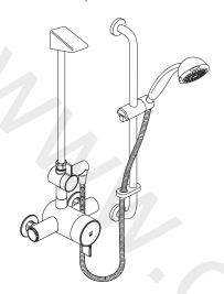
**Concealed Model:** This diverter is designed to be installed on the outlet of the Rada V12 Concealed Mixer. A flow regulator (6 and 9 l/min supplied with the Rada V12 Mixer) can be fitted to the right angled connector (RAC) if required.
