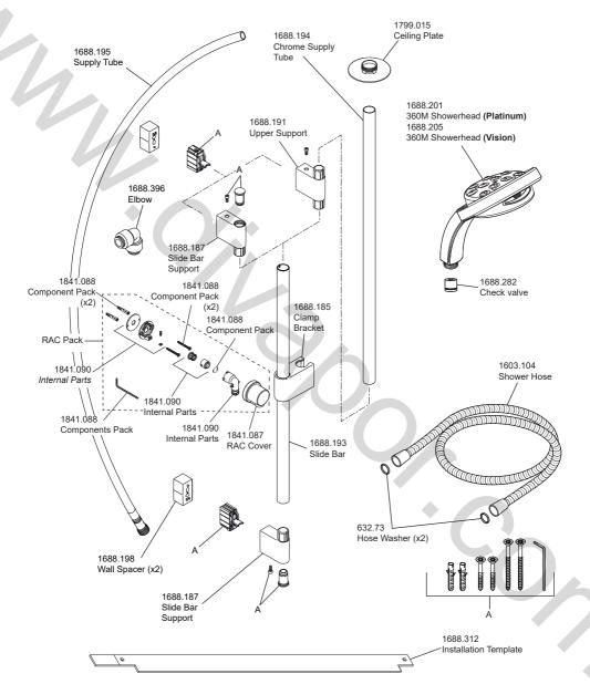
1688.184 Seal and Screw Pack - Components Identified 'B'. 1688.190 Classic Fittings Component Pack - Components identified 'A'.
