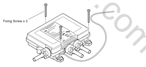
Drill and plug the fixing holes.
