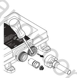
Refit seals and plastic nuts. Plastic nuts require hand tightening only.
