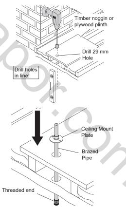
Centralise the brazed pipe in the hole then screw the ceiling mount plate to the wooden support.
