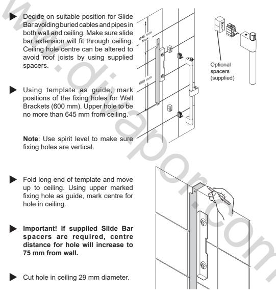
Drill and plug Slide Bar Assembly fixing holes.
