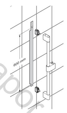
Insert fixing screws through holes in Wall Brackets and fix to wall. Do not fully tighten at this stage. Use template to set correct distances between Wall Brackets. Fully tighten screws.
