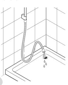
Press "o" button and reduce temperature to full cold "CLd". Increase to full flow. For Low Pressure (pumped) version, let shower run in order to prime the pump. For long pipe runs, allow 3 - 4 minutes for priming.
