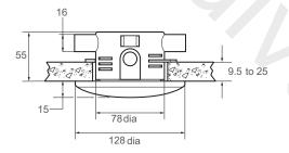
**Specify as: Mono-Control System MC126 (1.1495.013)** Each group of urinal bowls to be served by one Rada Mono-Control System MC126 ceiling mounted flow control. Complete with concealed passive infra-red sensor, control module and ½" solenoid
