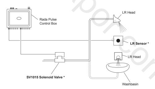
**Note!** Only the Sensor and Solenoid are supplied with this operating system as indicated \*
