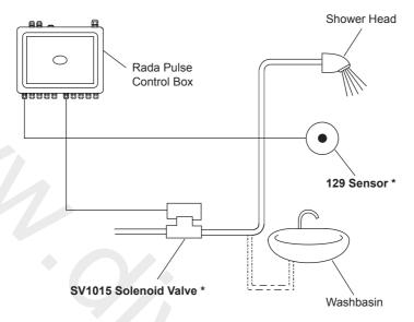
**Note!** Only the Sensor and Solenoid are supplied with this operating system as indicated \*
