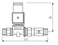
Specify as: Rada Pulse 129 Operating System (1.1495.068) Each outlet to be served by one Rada Pulse 129 Operating System wall mounted 'no touch' flow control. Complete with chrome plated active infra-red sensor and  $\frac{1}{2}$ " solenoid valve with isolator and filter.
