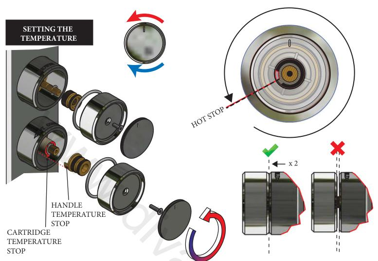
1. Assemble the Temperature handle to the Thermostatic cartridge.
