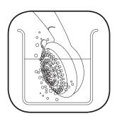
2. If scale deposits are stubborn, Soak the shower-head or hand-shower in a proprietary Limescale remover and rinse thoroughly before use.
