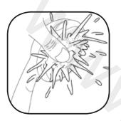
1. To break away scale deposite on a daily basis simply rub your thumb over the surface whilst the shower is running.
