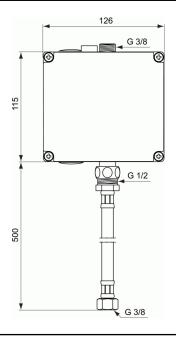
Basin electronic box KIT 1 / one valve / AC multi-box in connection with A3808NU Basin electronic box KIT 1 / one valve / AC multi-box in connection with A3808NU
