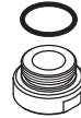
A6256AA Universal filter adaptor. Replaces the Armitage Bioguard outlet to permit attachment of an outlet filter. Threaded M24x1 (internal).
