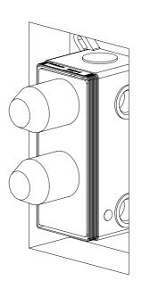
Board the wall, we recommend a suitable waterproof board is used and seal the edges of the Easi-Box.
