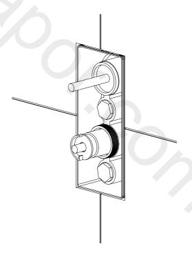
Trim away any excess from the lip of the Easi-Box using a sharp blade, ensuring that none of the lip protrudes beyond the finished wall surface.
