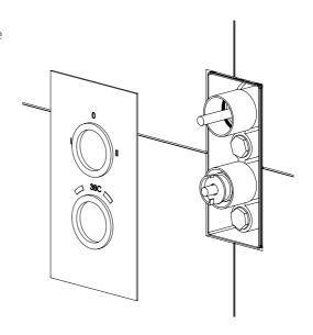
Fit the control knobs ensuring the stop pin of the temperature handle is located against the top of the stop ring.
