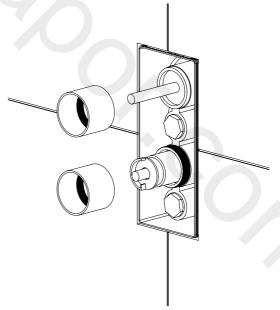
Apply a little silicone grease to the O rings of the fascia plate and a narrow bead of silicone sealant to the back and slide into place.
