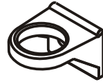
Fig 9 shower hose restraining bracket. Screw to the wall in a suitable position as shown below
