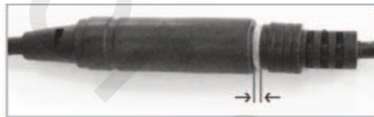
O-ring visible – not connected properly
