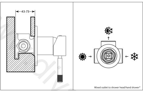
Install the concealed part at a depth so that finished surface is between the Min/Max markings shown above. Install the **cold** water supply from the <u>right</u> and the **hot** water supply from the <u>left</u> as per the above (*if possible pressure test*).
