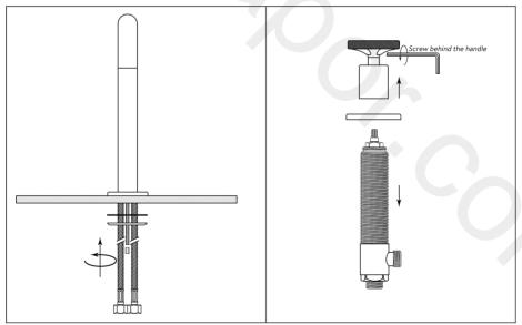
Slide the rubber 'C' washer followed by the metal 'C' washer and tighten the back nuts with a spanner to secure the spout.
