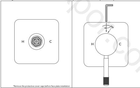
Apply the surrounding finishes, fit the face-plate onto the valve body.
