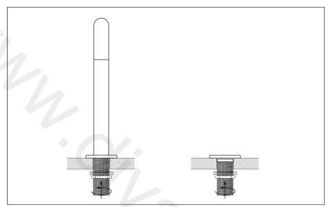
The spout and hand-shower holder can simply be installed by placing through and tightening with the washer and back-nut
