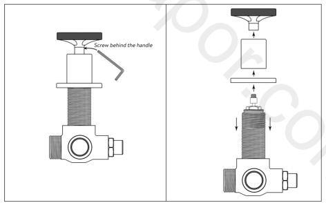
Installation of diverter. Loosen the screw (behind the handle knob) with an allen key. Seperate the diverter knob, base plate and shroud from the valve body.
