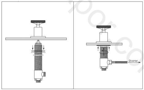
Screw the back-nut, metal washer and rubber washer down the valve body. Install the valve from underneath and secure with the base plate and handle.
