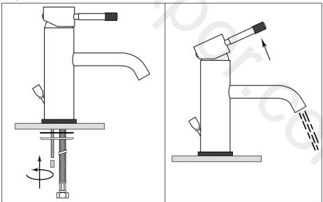
Slide the rubber 'C' washer followed by the metal 'C' washer and tighten the back nuts with a spanner to secure the mixer.
