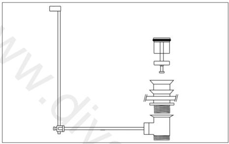
Dissemble the pop-up waste and reassemble onto the basin ensuring the foam washer is placed between the top waste housing and the basin. The rubber washer is to be placed on the bottom waste housing before being tightened
