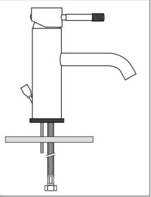
Install the threaded rods and **hand**-tighten the flext-pipes into the bottom of the mixer body. Feed the assembly through the hole in the basin/countertop.
