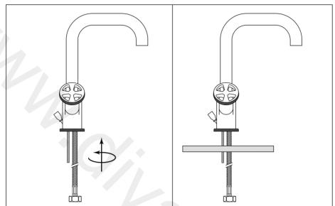
Install the threaded rods and **hand**-tighten Feed the assembly through the hole in the the flext-pipes into the bottom of the mixer basin/countertop. body.
