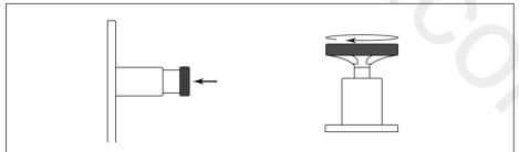
All diverters only function when the main water supply is turned on, for concealed shower valves push the button in to divert and for deck/floor mounted bath/shower mixers pull the diverter knob
