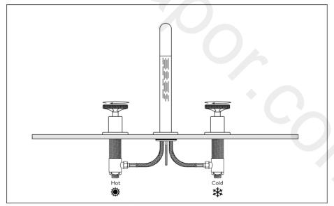
Flush the pipework then connect the flexi-pipes to the isolation valves, turn on the water, run the tap and check for leaks.
