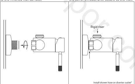
Install the washers/filters in to the mixer body, then hand tighten the mixer to the eccentrics, ensure its level. Place a cloth over the nuts to protect from scratching when fully tightening with a spanner. Turn on the water and test.
