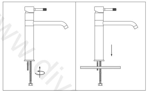
Install the threaded rods and **hand**-tighten Feed the assembly through the hole the flexi-pipes into the bottom of the mixer in the kitchen sink/countertop. body.
