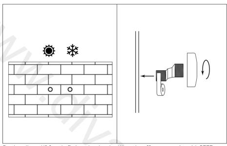
Pre-Install two ½" female fittings, level and 150mm apart, these fittings must be flush to the finished wall surface.
