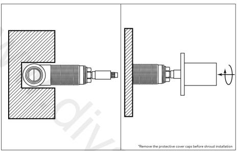
Install the concealed part into the wall and connect the water supply (*if possible pressure test*).
