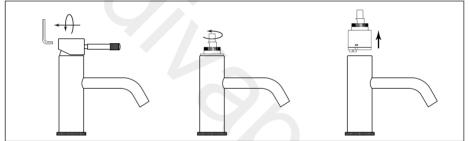
Remove the push cover. Using an Allen key loosen the grub screw this will allow the handle to be removed. Unwind the shroud, Care-fully with a spanner loosen the locking nut, this will allow the cartridge to be taken out and replaced. When inserting the new cartridge make sure the 2 locating points align, then re-assemble.
