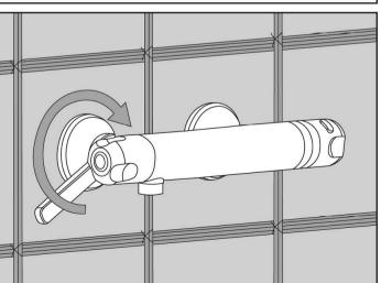
We recommend that the pipe work is well flushed through before installing the bar shower mixer to prevent debris damaging the mixer.
