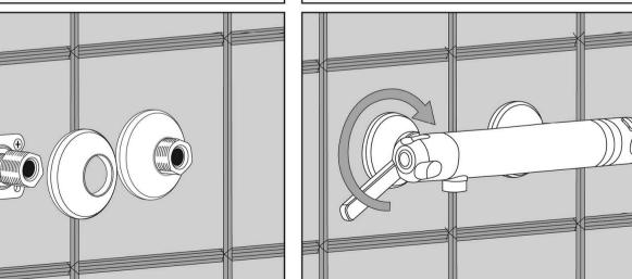
Spin the chrome plated covers on to the hexagonal collar and the connections are ready for the installation of the bar
