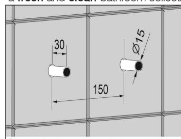
Ensure existing 15mm copper supply pipes are at 150mm centres and protrude from the tiling surface by 30mm.
