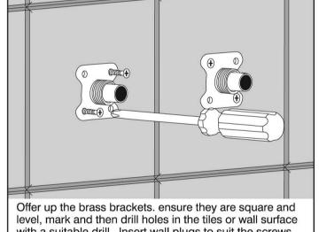
with a suitable drill. Insert wall plugs to suit the screws you have chosen (not supplied). Fix the brackets in place with at least two screws in each (preferably four in each).
