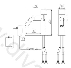
Power supply  $6 \times 1.5 V$  AA Battery or 9V transformer
