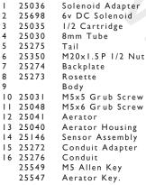
N.B. For replacements 1&3 come as an assembly Part No. 25655
