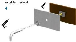
Fit Splashback with adhesive (or other fixing method as required) leaving mounting assembly protruding
