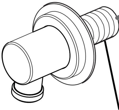
Cut to length if required. Threaded joint connections should be made with PTFE tape. Oil based, non setting jointing compounds should not be used.
