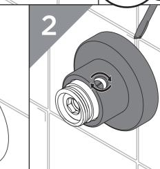
Rotate the shroud until the opening aligns with the isolation screw.
