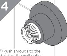
back of the wall outlet. securing them against the rubber fixing plate
