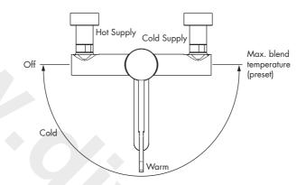
As the handle is rotated anti-clockwise from the off position the delivered water progresses from cold, through warm to the pre-set maximum temperature of approximately 43°C.
