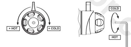
Turn the temperature control back to the maximum hot setting and measure the outlet temperature, when stabilised with a calibrated thermometer.
