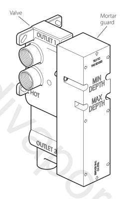
Rinse pipe work thoroughly before fitting the valve: do not allow dirt, metal particles or shavings to block the filters fitted on inlets.
