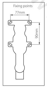
Select the position for the shower valve and offer the shower valve to the wall, make sure the valve is vertical with a level and mark the 4 fixing points with a suitable pencil, see above right for dimensions. Remove the shower valve from the wall, drill the holes to a suitable depth for the wall plugs and secure with suitable screws.
