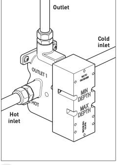
Finish the wall by tiling up to the mortar guard, keep the final finished wall surface between the min and max marks.
