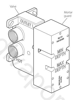
Rinse pipe work thoroughly before fitting the valve: do not allow dirt, metal particles or shavings to block the filters fitted on inlets.
