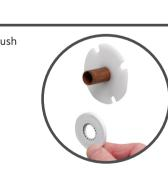
Trim the projecting pipe to a length of 15-22mm, measured from the face of the gripper ring, using a suitable cutter. If a hacksaw is used, the pipe end must be carefully de-burred and chamfered.
