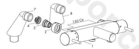
Note: The deck mounting legs are supplied complete with retaining nuts.
