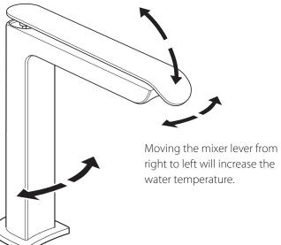
The whole mixer/spout can be swivelled to the left or right accordingly.
