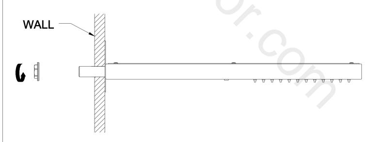
3. Fix the two inlets through the wall. Tighten the backnuts and connect the hoses.
