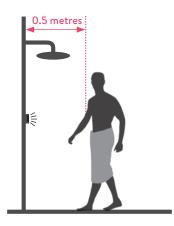
The proximity sensor detects any object directly in front, at approximately 0.5m away from the controller. See page 17 for more information.
