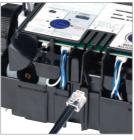
A further data cable socket has been provided for use with the secondary Digital remote control or Digital diverter. This can be accessed by carefully snapping and removing the
