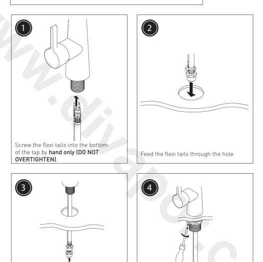
Slide the rubber and metal washers onto the thread and secure in place by tightening the backnut up to the underside of the basin. The screws on the backnut allow for any uneven surfaces and should be tightened up to the metal washer.
