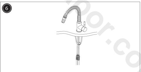
Connect the flexi tails to the hot and cold water supplies. Turn on the mains water supply letting the water flow for a minute to flush through the system. Check all joints and connections for any leaks.
