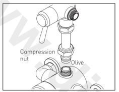
I. Push the short connecting tube into the top outlet on the shower valve (not supplied) ensuring the nut and olive are fitted to the connecting tube. Tighten the compression nut fully using a suitable spanner.
