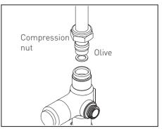
2. Fit the Rigid riser to the diverter valve. Tighten the compression nut fully using a suitable spanner to ensure a water tight seal.
