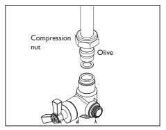
2. Fit the Rigid riser to the diverter valve. Tighten the compression nut fully using a suitable spanner to ensure a water tight seal.
