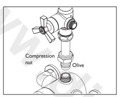
I. Push the short connecting tube into the top outlet on the shower valve (not supplied) ensuring the nut and olive are fitted to the connecting tube. Tighten the compression nut fully using a suitable spanner.
