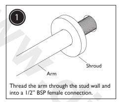
Secure the arm in position by tightening the clamp and backnut. The supply pipework to the shower valve must be rigid and secured in position with the use of pipe clamps.
