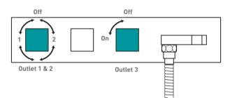
Turning the flow control in the direction of the arrows increases the flow of water to the outlets.
