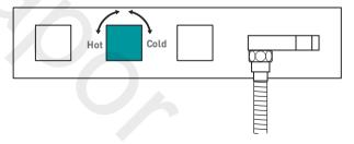
Turning the temperature control handle in the direction of the arrows increases/decreases the temperature
