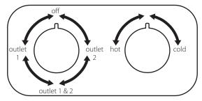
Turning the right handle anti-clockwise will increase the water temperature.
