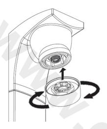
2. Invert the spray plate holder and use to unscrew the locking collar.
