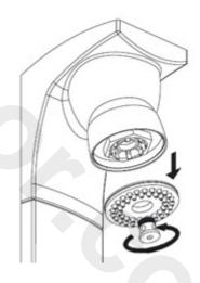
1. Unscrew the locking screw using a 4mm hexagonal key and remove the spray plate and spray plate holder.
