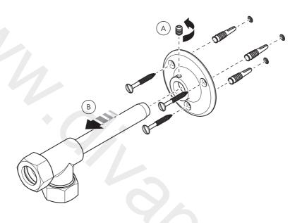
Please note that pipe connections to the riser pipe bracket are made using compression nuts and Ø19mm olives (supplied). Please refer to 'Connections' in the 'Important Information' section.
