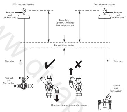
Diverter connections are compression nut and Ø19mm olives
