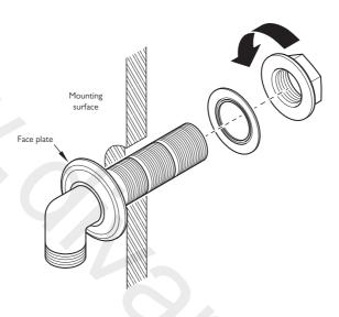
Note: Before fitting the wall outlet ensure that a rubber 'o' ring is fitted to the rear of the face plate. This is factory fitted, though may have worked loose during transit.
