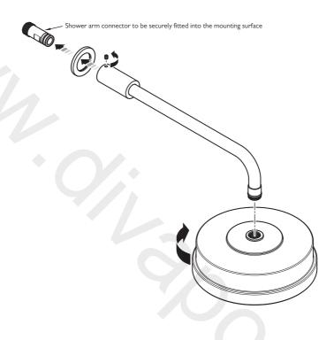
I To aid installation the shower rose and arm can be disassembled as shown above. Ensure that the set screw is removed completely to avoid damage to the 'o' rings. The set screw can be removed using a 2.5mm hexagonal key.
