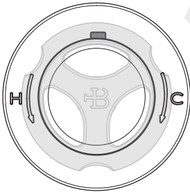
Safe temperature button set to top (suitable for right and left handed operation)
