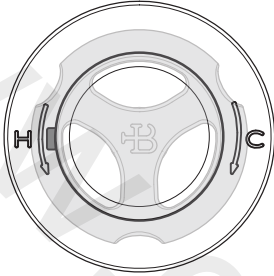
Safe temperature button set to left (suitable for right handed operation)
