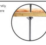
The minimum height required behind the ceiling is 50mm and the space must allow for an 80mm wide, 50mm deep noggin to be used to support the assembly.
