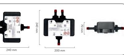
solation valves are supplied with the Aqualisa SmartValve™ and diverter (where supplied) and must be fitted on all inlet and outlet connections. All connections require 15mm pipe, and all pipe work should be supported.
