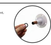
The 'O' ring must be positioned on the 15mm pipe flush to the fixing bush, not onto the
