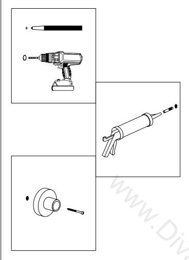
Drill the screw holes and install the wall plugs. To create a seal, apply a small amount of silicone on the inside of the wall plug. 8
