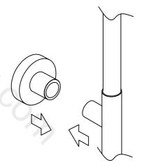
Fit the wall bracket to the riser kit
