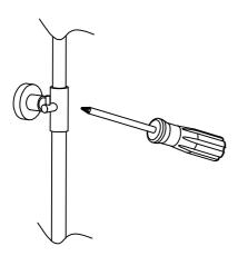
Make sure the riser is level, mark the position of the screw holes on the wall bracket. 6
