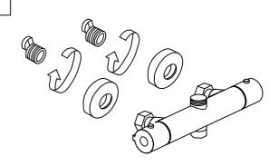
Fit decorative covers over the offset connectors. Then insert sealing washer into nut and tighten onto offset connectors with wrench, being careful not to damage the chrome finish on the connecting nuts.
