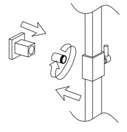
Install the riser into the top outlet of the shower valve.
