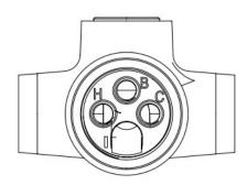
Feed the tails throught the barrel thread and hand tighten into the tap. Fit the tap in the desired location using the locking nut and accompanying screws.
