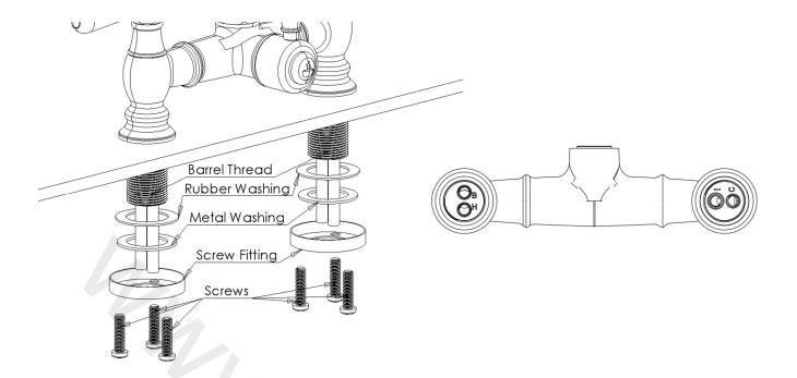
Feed the tails throught the barrel thread and hand tighten into the tap. Fit the tap in the desired location using the locking nut and accompanying screws.
