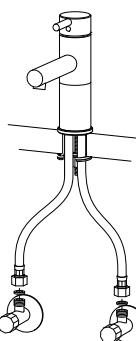
4. Connect the two flexible hoses with the cold and the hot water inlets to the relevant water supply. For a seal there must always be a washer in the floating nut on the end of the flexible connectors.
