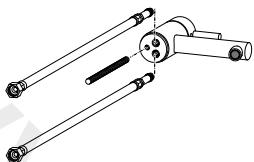
1. Screw the two flexible connectors into the holes provided. Screw the threaded rod in the hole provided in the body of the tap.
