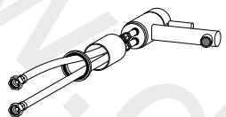
2. Pull the shaft and the base ring over the tubing and threaded rod for fitting.
