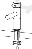
3. Locate the tap into the hole provided in the sink/countertop. From the underside slide the crescent gasket and the metal disk onto the threaded rod, tighten the fitting using the brass-coloured locking nut.
